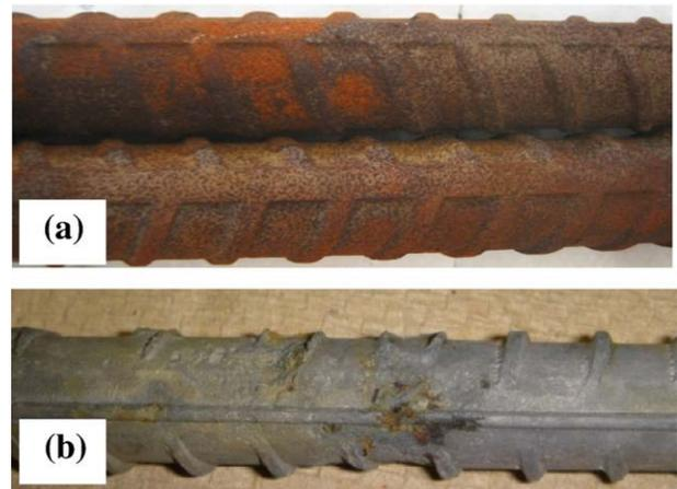
Fig. 2. Distribution of the corrosion products on the surface of the steel rebar: (a) due to impressed current which occur over the whole surface [61] and (b) due to natural corrosion which is localised [62].
