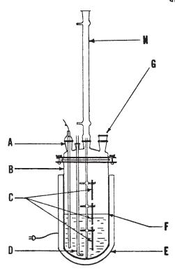
Note 1—The flask can be used as a versatile and convenient apparatus to conduct simple immersion tests. Configuration of top to flask is such that more sophisticated apparatus can be added as required by the specific test being conducted. A = thermowell, B = resin flask, C = specimens hung on supporting device, D = air inlet, E = heating mantle, E = liquid interface, E = opening in flask for additional apparatus that may be required, and E = reflux condenser.
