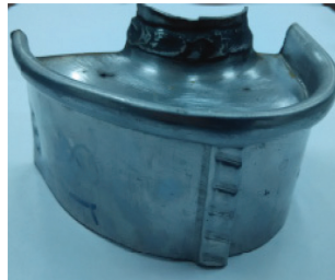
Figure 4. The end part of the front muffler A.
